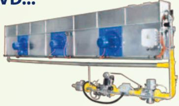
Traditional gas burners for direct fire in vertical dryers. With this type of combustion, the process air for drying, generated by the dryers fans, the combustion air generated by the burners fans and the combustion fumes, all mix together to form the air necessary to dry the product, reducing energy consumption. Heat capacity from 814 kW to 8150 kW.
