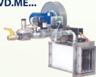
If in the VDPE series, the combustion body is inserted inside the channel of the air to be dried, this series has all its components on the outside of the channel. Only the flame enters into the channel and the combustion fumes. The burner has to be fixed to the channel with a steel flange, supplied. Heating capacity from 70 kW to 756 kW.
